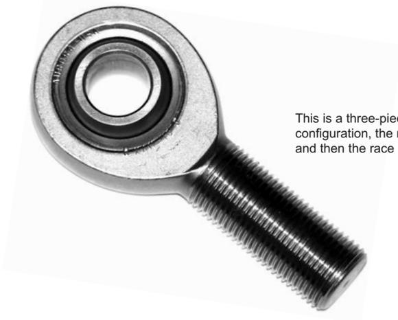
This is a three-piece ("aircraft") rod end. With this configuration, the race is formed around the ball, and then the race insert is staked into the body.
