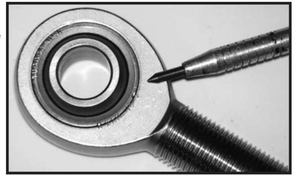
Because of the three-piece configuration, various materials can be used in the construction of the rod end. This process allows the rod end to best match the application (which often boils down to strength versus load).
