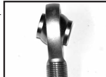
Misalignment is the degree of angular movement that a ball or sphere can accommodate without interference. This is a special "high misalignment" bearing (note the larger shoulder).
