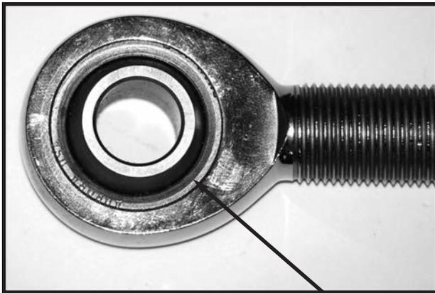
The rod end shown here incorporates a composite Teflon liner. You can purchase two or three piece rod ends with Teflon liners. The Teflon liner is bonded to the race so that the ball actually rides on the liner. The movement of the ball rubs Teflon on the ball, which in turn provides the necessary lubrication.
